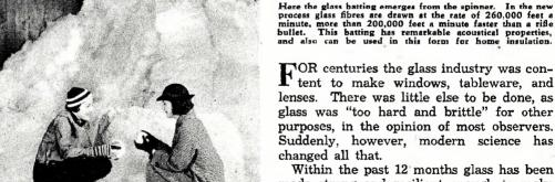
This is not snow but glass, the same kind from which bottles are made. One pound of this substance contains enough fibres to reach around the world. Each strand is 1/20th the diameter of a hair; 100 are needed to make No. 50 thread.
