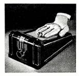
This new machine measures the palm and finger length to fit glove, with scientific accuracy.
