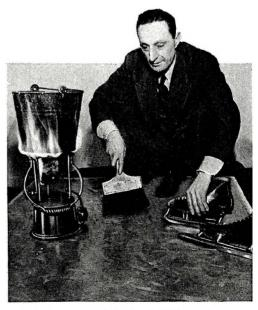
Applied to any surface in boiling liquid form this chemical ice hardens in a few hours leaving a skating rink equal to one of actual ice. The chemical may be reheated and used again.
