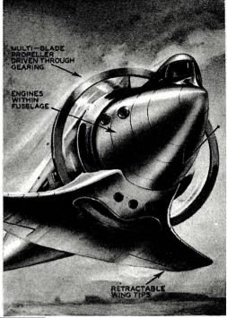
With wings reduced to a minimum this transoceanic plane is planned to span the Atlantic in five hours. In place of numerous motors blanketing over-sized wings, this craft uses a single power plant installed in the hull to drive a series of small, variable pitch blades constantly revolving about the circular ship.
