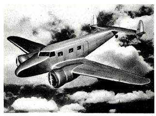
This is the new Lockheed 12 designed for small airlines, private industries, and as a feeder plane for the major sirlines. It carries 6 passengers, 2 pilots, and a 450 pound cargo at speeds up to 231 miles per hour.
