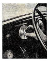
Trailer brakes can be adjusted according to the load weight with this simple dashboard control.
