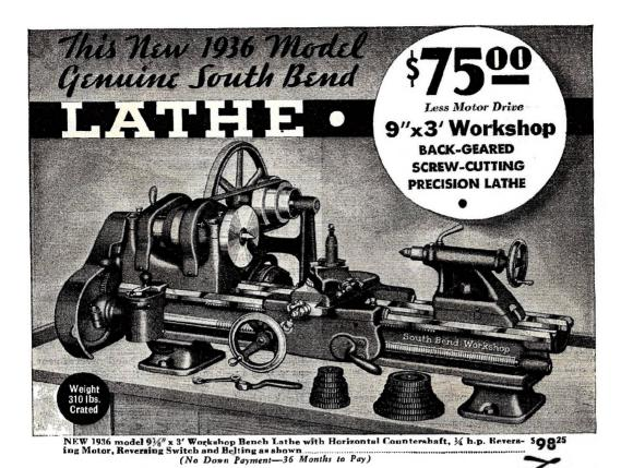
THE new 1936 model 9-inch Workshop Lathe swings  $9\frac{1}{8}$  over bed and  $5\frac{1}{2}$  over carriage. The hole through spindle is  $\frac{3}{4}$  and will accommodate collets up to  $\frac{1}{2}$  capacity. The 3-foot bed size takes 17" between centers. Screw three cutting range is 4 to 40 per inch right or left hand. Turning feeds as fine as .003" are provided for. Other bed lengths available are  $3\frac{1}{2}$ , 4' and  $4\frac{1}{2}$  at slightly higher prices.
