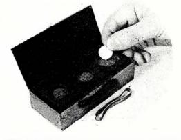
Wite the "Black Chamber Box" in the manner shown above. Use heavy wire for supporting flashlight bulbs and solder all connections well. Battery is glued to back of wood panel.
